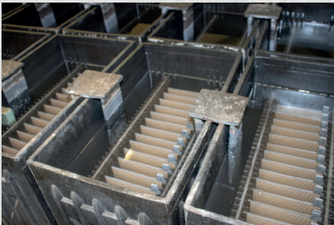
Individual battery plates are placed in the formation trays
